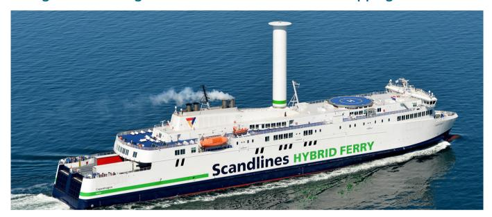
Norsepower is at the forefront of emerging clean tech for the shipping industry. Their Rotor Sail is the first proven auxiliary wind propulsion system that enables cargo, cruising and other shipping vessels to reduce fuel consumption by augmenting their power systems.
