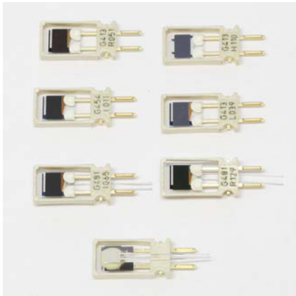
Family of HUMICAP sensors
