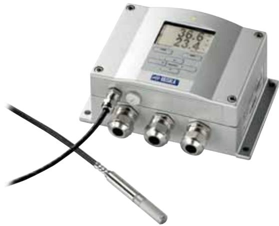
*Vaisala HMT330 series transmitters deliver high accuracy and excellent long-term stability. RH accuracy is within 1% up to 90% RH and within 1.7% up to 100% RH. Temperature accuracy is within 0.2°C (0.36°F).*
