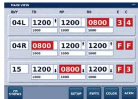
*A customer-specific controller's display was designed for the FAA Runway Visual Range System using Vaisala AviMet's new display development tools.*
