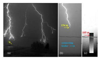
Fig. 8. Images of attachment processes for first and subsequent return strokes in natural lightning (Figure c is a regional contrast-modified image of Figure b, with the color-reversed connecting leader of subsequent return stroke) [Adopted from Jiang et al., 2015]
