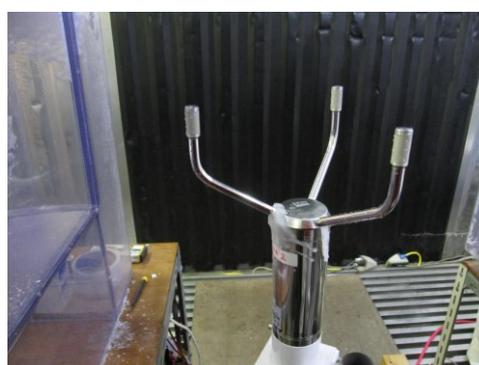
**Figure 7.** New sensor design was operative throughout the test period with the icing test profile (Table 3).
