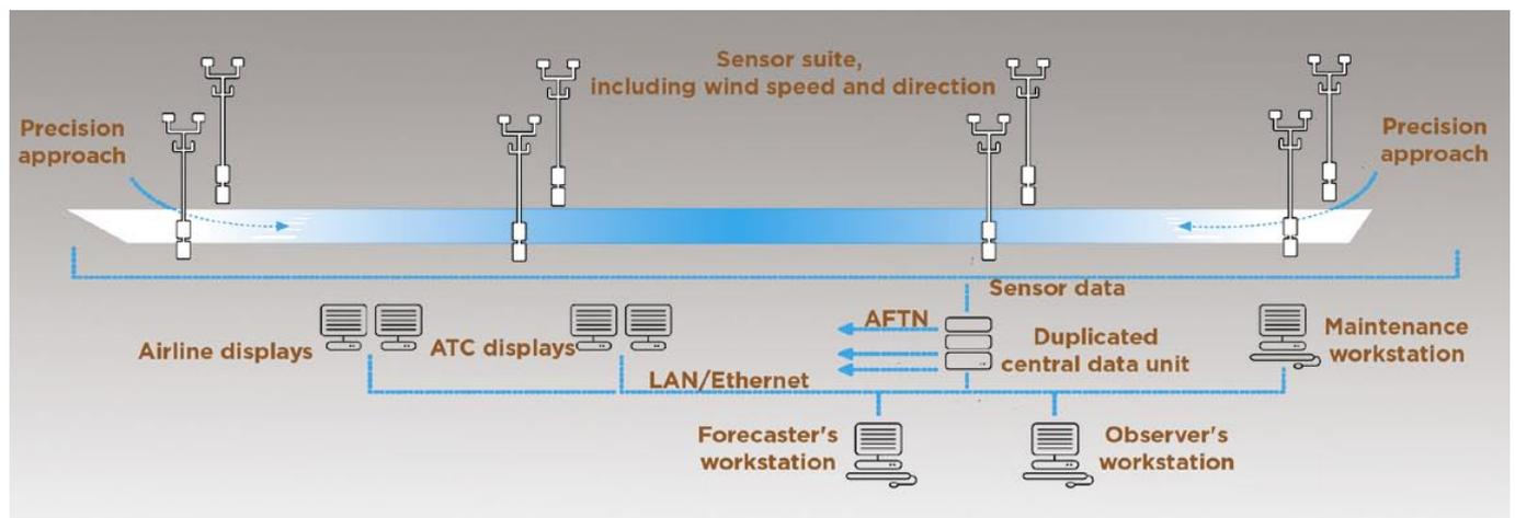
Fig. 4 A typical LLWAS consisting of field sensors, central data unit(s), communication interfaces and different workstation types.
