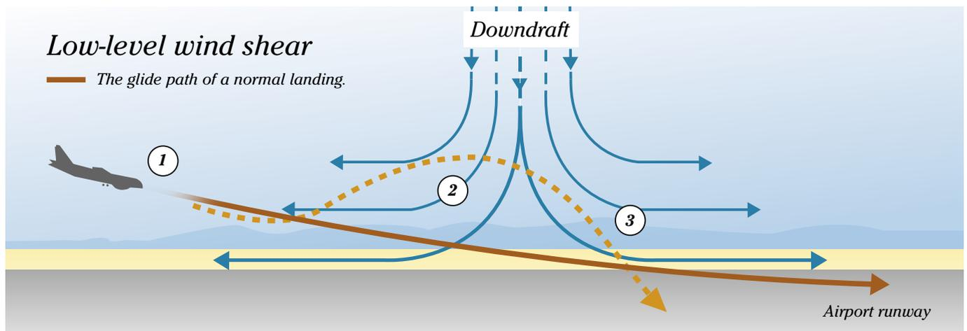
**1.** A headwind slows and lifts the aircraft above its normal flight path. **2.** While the pilot compensates for the headwind by dipping the nose, the aircraft enters a downdraft. **3.** A tailwind dangerously reduces the aircraft's speed.
