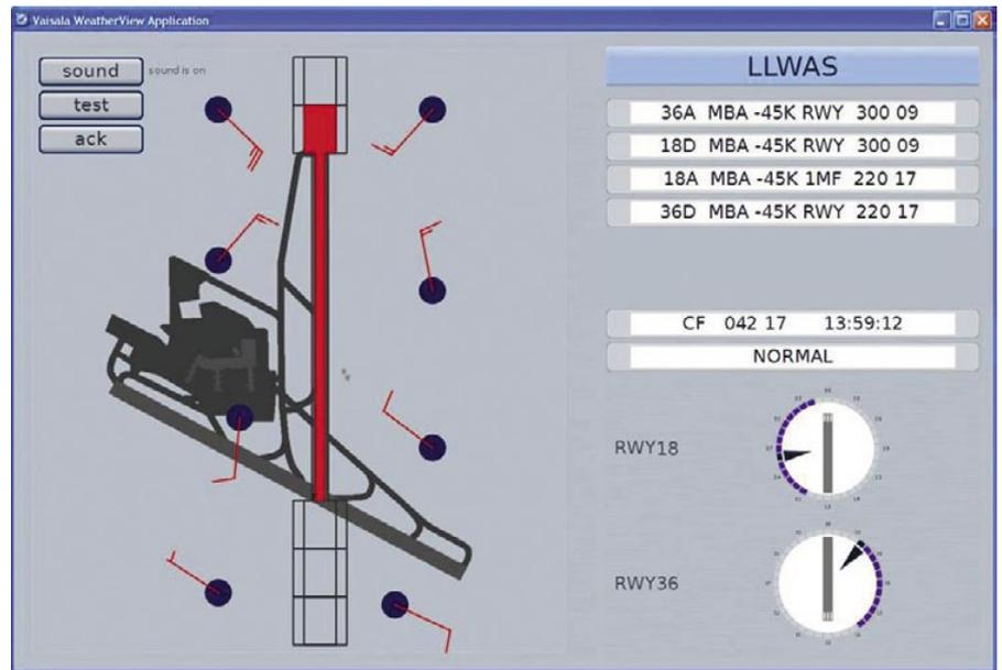
Fig. 5 An LLWAS display showing the sensors and wind shear information.
