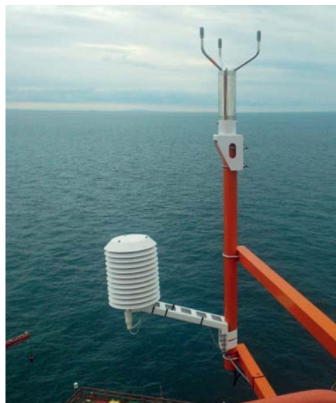
Ultrasonic Wind Sensor and Humidity and Temperature Probe installed on offshore platform (photo: Vaisala Maritime)
