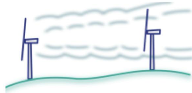
(b) Turbulence generated by turbine wake
