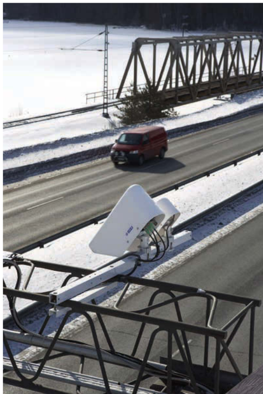
(Left) The remote sensor measures surface temperature via emitted infrared radiation and lasers
