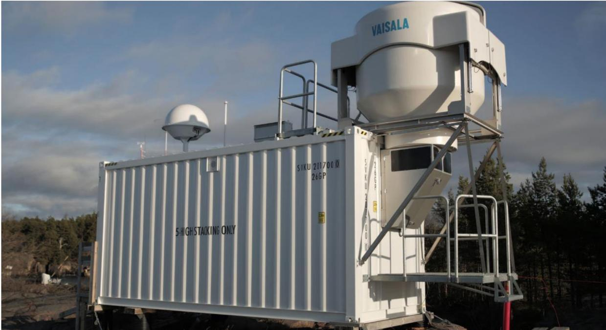
An automatic sounding system makes the sounding process efficient and reliable.
