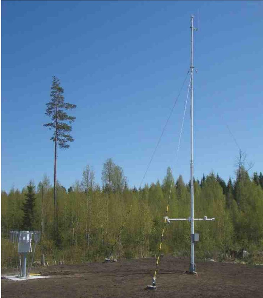
A 10 m mast with meteorological sensors at Metsähovi research station.
