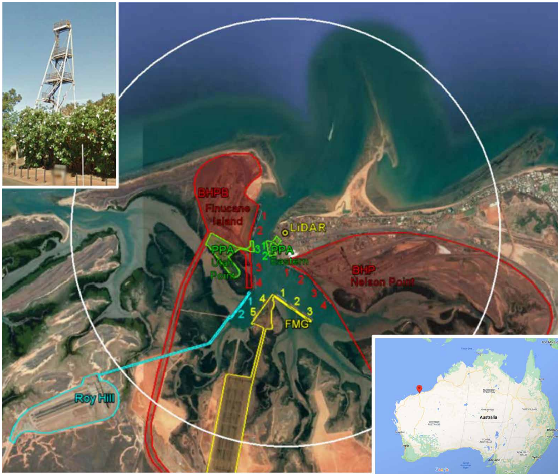
LEFT Port Hedland outlining industries and players currently using the port to export commodities such as BHP, Fortescue Metals Group Limited (FMG), Roy Hill, Pilbara Ports Authority (PPA) and Dampier Salt. The five-kilometre radius white circle is centered on the LIDAR location atop the Town Centre Viewing tower (inset) and represents the approximate coverage of the LIDAR beam.
