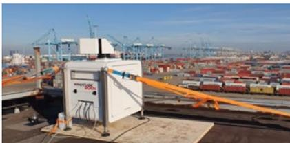
**WindCube® Scan lidar** providing 3D, spatial wind data at ranges even beyond 10km
