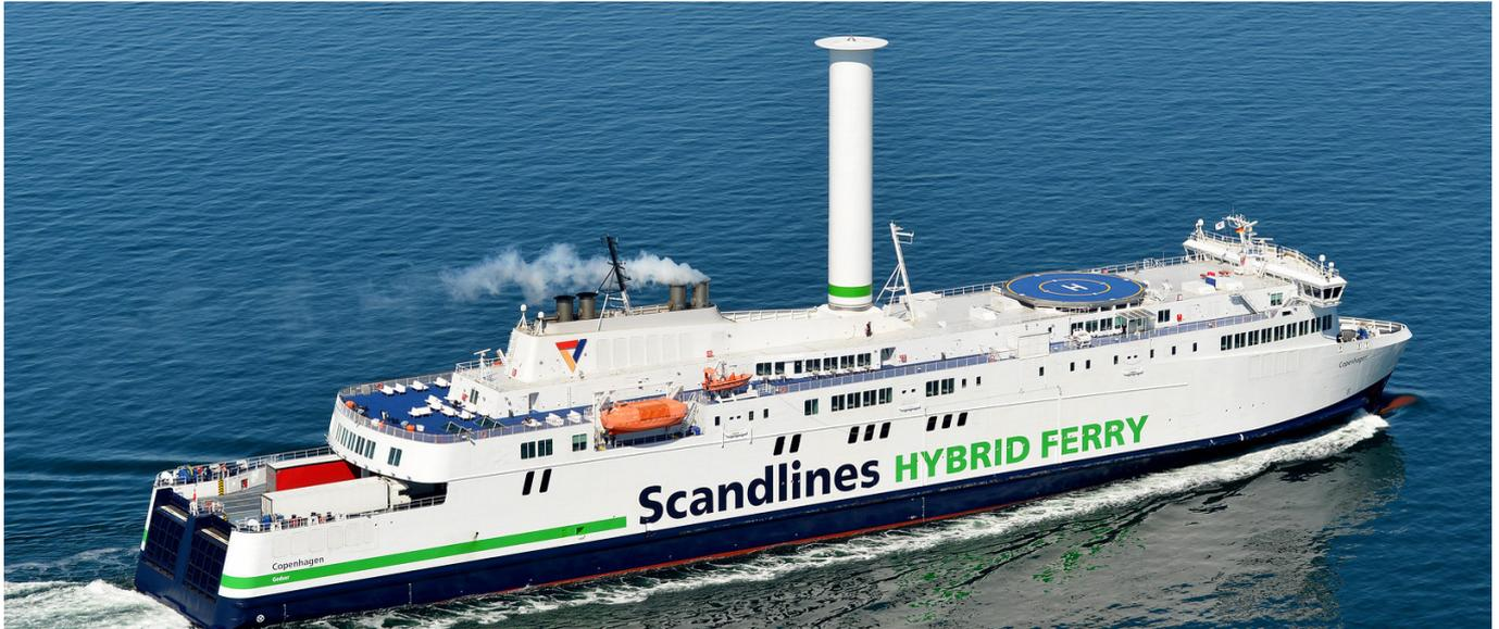
*Norsepower is at the forefront of emerging clean tech for the shipping industry. Their Rotor Sail is the first proven auxiliary wind propulsion system that enables cargo, cruising and other shipping vessels to reduce fuel consumption by augmenting their power systems.*
