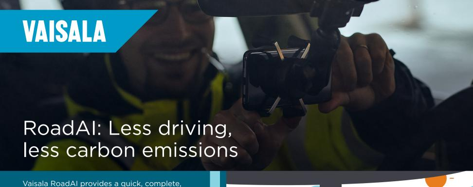
objective analysis of pavement conditions through an automated road survey methodology. Gathering video with a smartphone attached to any vehicle, the solution identifies road conditions across the full road width plus defect types and repairs, creating multiple datasets that provide actionable information for planned and reactive maintenance — all from the same drive.
