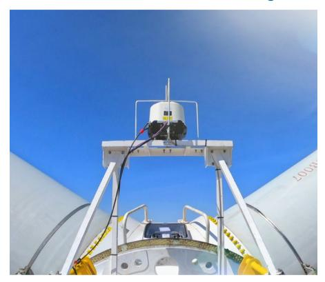
WindCube Nacelle makes Lidar-Assisted Control (LAC) a reality, reducing Levelized Cost of Energy (LCOE) and creating numerous other benefits for wind energy.
