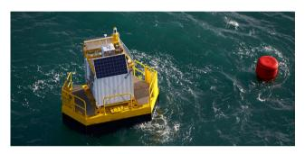
WindCube Offshore equips the WindCube vertical profiler with a robust casing for integration into floating buoys and other harsh offshore locations, such as lighthouses, substations, and vessels.
