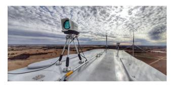
Suitable for any turbine type and rotor diameter, WindCube Nacelle provides a complete picture of the wind profile at unprecedented ranges from 50 to 700m (long-range version).
