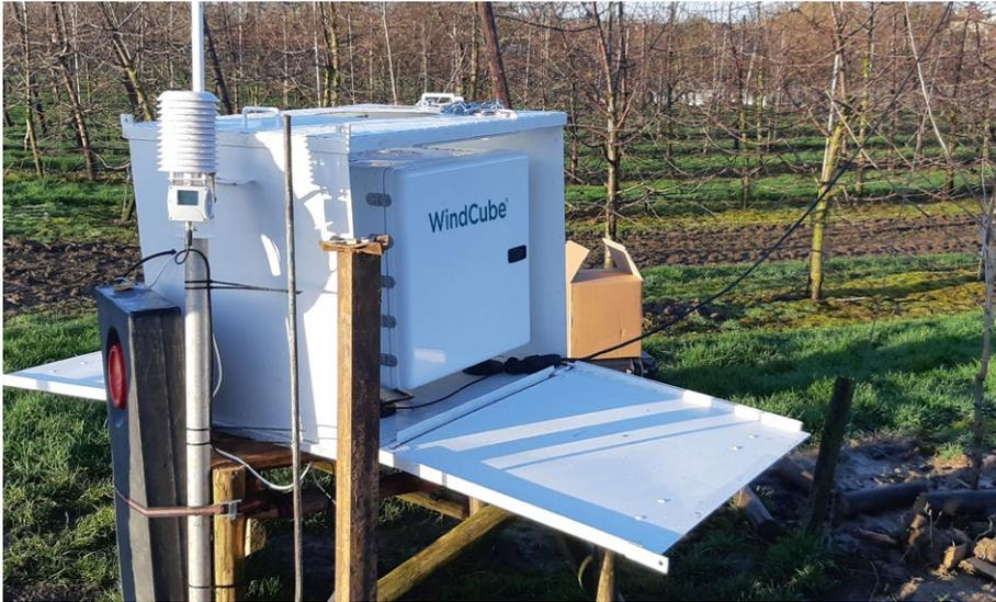
“Overall, better accuracy classes than evaluated for WindCube v2.1 in the height range above 100m can hardly be expected for any monostatic remote sensing devices implementing probe volume spatially separated by about 50m to 150m for detecting different radial wind speed components.”
