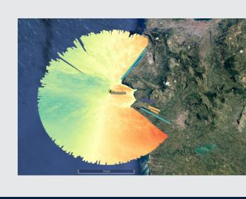
wind across 360° using several scanning patterns, up to ranges of 15km and beyond. This capability is useful for many onshore and offshore projects. Scanning lidar provides full 3D wind awareness, even
