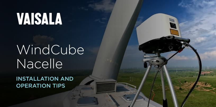
WindCube Nacelle lidar enables developers and operators to efficiently and accurately assess and verify performance to ensure maximum power output. Classified according to the IEC 61400-50-3 standard, it is widely accepted for contractual and operational Power Performance Testing (PPT), both onshore and offshore, and is increasingly included in manufacturer Turbine Supply Agreements (TSAs) to verify offshore turbine installations.
