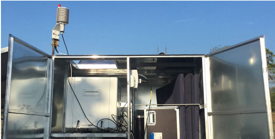
WindCube installed inside of a trailer designed by Ventus
