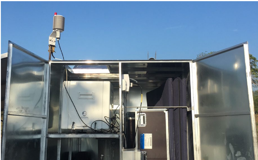
WindCube installed inside of a trailer designed by Ventus
