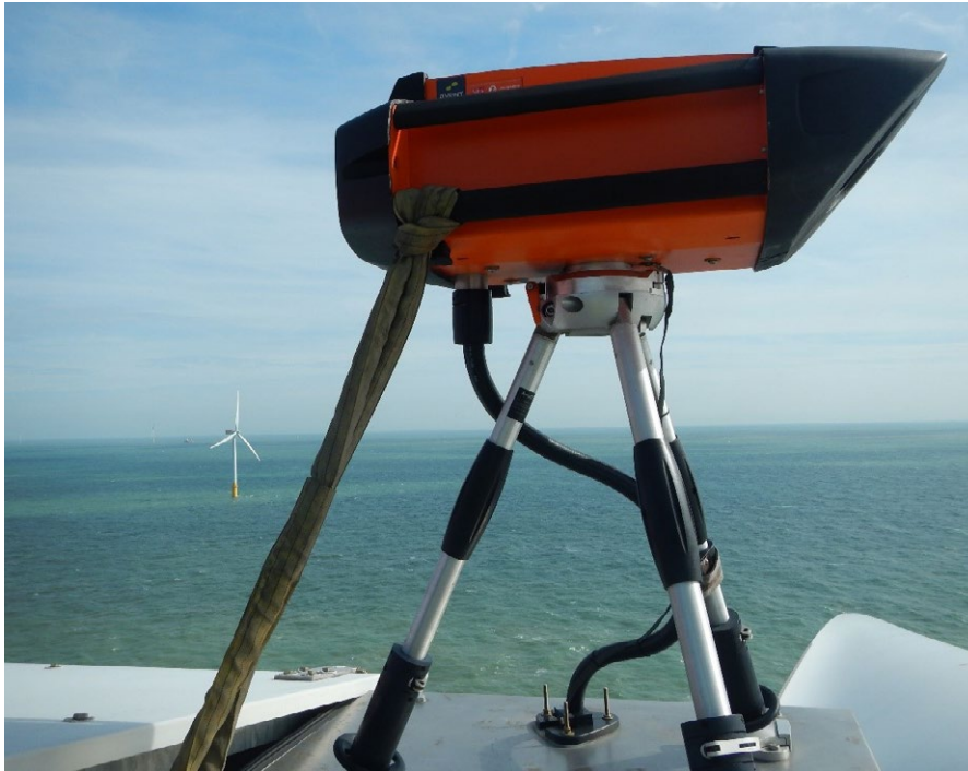
Installation of Wind Iris 2-beam (earlier version of current WindCube Nacelle) by SSE
