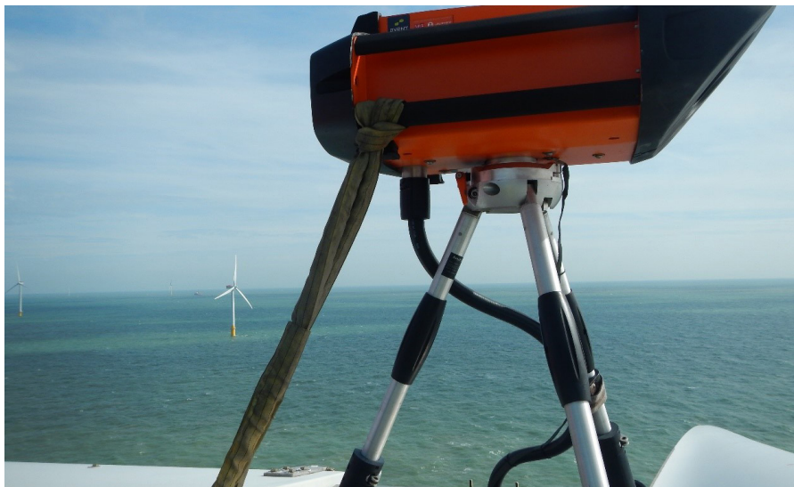
Installation of Wind Iris 2-beam (earlier version of current WindCube Nacelle) by SSE
