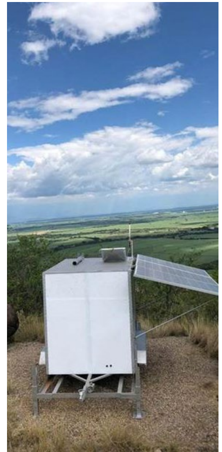
WindCube lidar in trailer.
