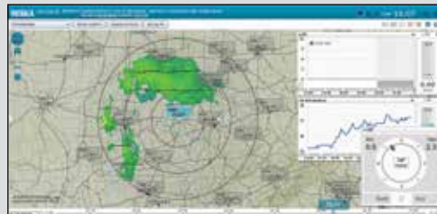
View 2 – When viewing the same storm through Vaisala's AviCast single site radar it depicts a more accurate view. Precise size and location of the storm north of SDF airport with no precipitation forecast to occur at the airport.
