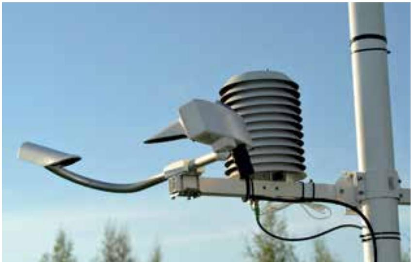
validated data that can be visualized using the optional Vaisala MCC301 PC display software. In its pre-configured setup, the customer may choose from a range of sensor options to measure air temperature and humidity, barometric pressure, wind speed and direction, precipitation amount, solar radiation, present weather and
