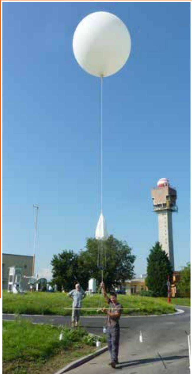
In each sounding there were used 4 radiosondes - two of RS41 and two of RS92. Sondes were hanging about 60 cm under wooden cross-rod, so they made corners of square with a side of about 1,5 m. The cross-rod itself with parachute was about 50 meters under the balloon. Data from both RS41 were processed with MW41 system while one of RS92 was processed with MW21 and the other
