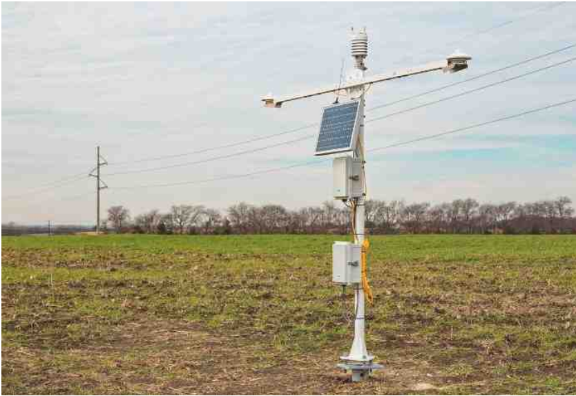
Vaisala Solar Weather Station SP12 is an all-in-one system specifically designed for the solar industry to help collect reliable ground measurements.
