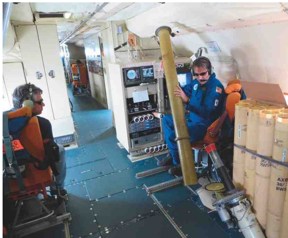
NOAA Aircraft Operations Center technician, Mr. Damon Sans Souci, preparing to launch an expendable into a storm from the WP-3D Orion Hurricane Hunter.
