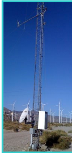
A Vaisala AON system in San Geronio Pass near Palm Springs, California. Wind speed, wind direction, and temperature are measured at 10 m and 30 m above ground level to improve Southern California Edison's wind power forecasts provided by AWS Truewind. The Shell WindEnergy Whitewater Hill Wind Park's GE 1.5 MW turbines are visible in the background.
