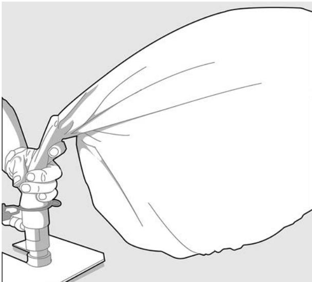
6. When the balloon is sufficiently filled, in other words, the balloon just raises the gas nozzle, close the gas valve.
