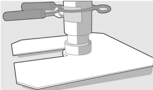
4. Secure the neck of the balloon to the balance nozzle with a clamp as shown in the figure below. Look out for sharp objects near the filling balance so that no damage is caused to the relaxed balloon.
