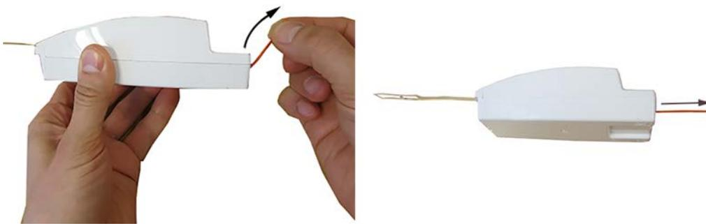
Before you launch the radiosonde, you can return to the preparation phase by releasing the strap around the radiosonde. The sounding software automatically returns to the ground check phase.
