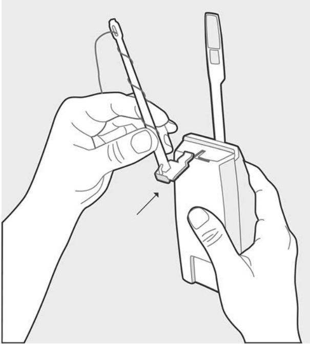
2. As you push, the unwinder stick pushes the sensor boom to the bent position and the unwinder snap lock clicks into place.
