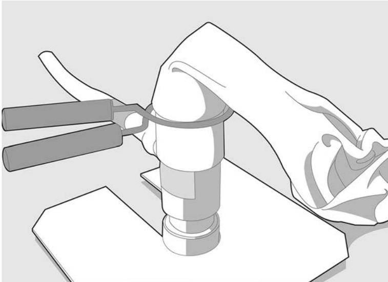
5. Turn on the gas from the pressure reducing valve. Let the gas flow slowly into the balloon. Do not leave the balloon-filling shed while inflating the balloon. Follow the balloon manufacturer's instructions when inflating the balloon.
