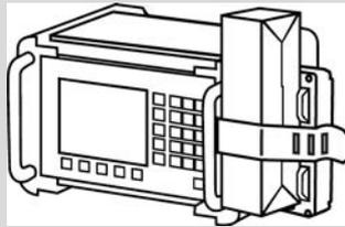
4. Attach the radiosonde to the unwinder.
