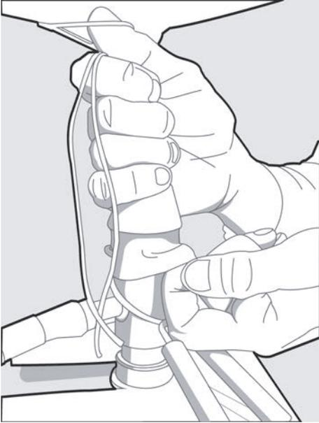
9. Fold the neck of the balloon over and secure firmly. Cut off any extra string. The figure below shows an example of a secured balloon neck. In the figure, the balloon is attached to a balloon holder hook.
