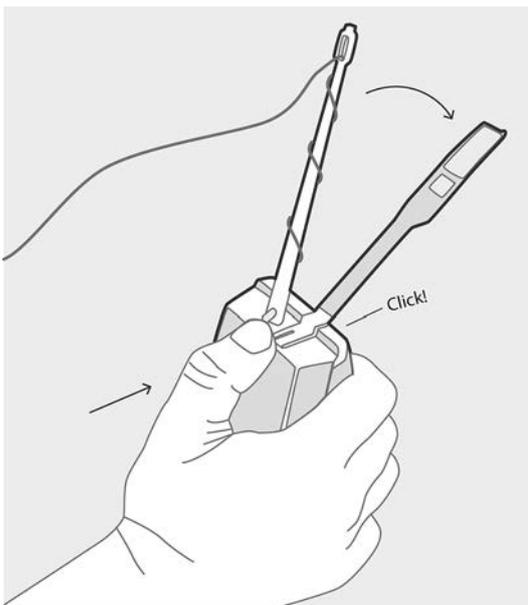
3. Make sure that the unwinder is firmly attached to the radiosonde.
