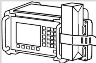
3. Pull the strap over the radiosonde. The radiosonde is switched on automatically. The sounding software automatically detects the radiosonde and begins the sounding preparations.
