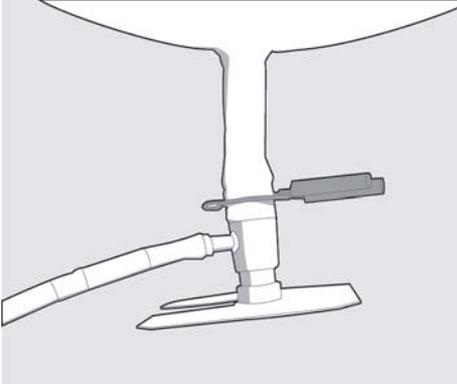
7. Before removing the balloon from the gas nozzle, tie the neck of the balloon tightly above the balance nozzle with approximately 0.5 m (2 ft) bit of string.
