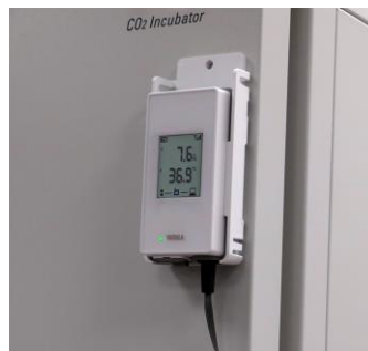
Continuous monitoring Easy use of wireless data loggers with CO 2 measurements, improving CO 2 monitoring in life science GMP251 + RFL100 data loggers
