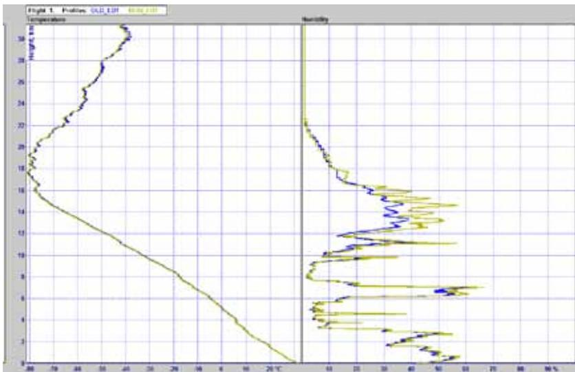
*A day-time sounding profile from Malaysia, showing the effects of the improved algorithms on the humidity and temperature measurements.*
