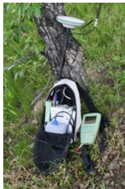
Equipped with a single transducer, the Vaisala BAROCAP® Digital Barometer PTB220 is packaged in a compact backpack along with the GPS receiving equipment and power supply.
