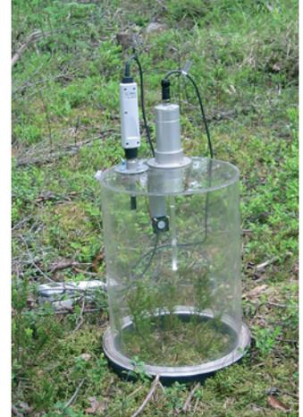
Figure 1. The soil respiration chamber and the measurement set up for the trial measurements conducted at the Hyytiälä Forestry Field Station in Hyytiälä, Finland.
