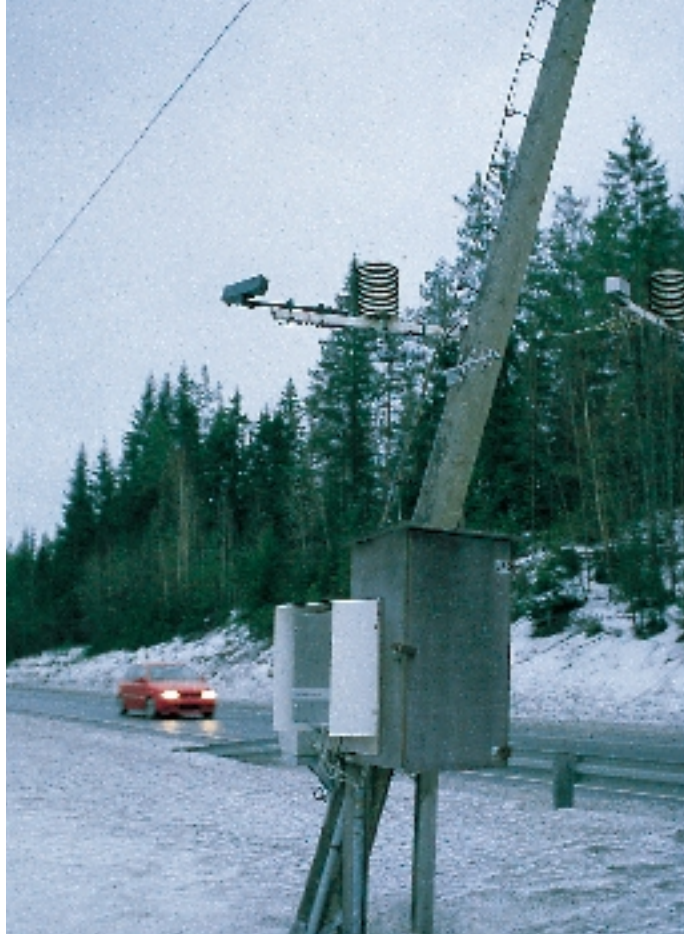
Finnra tested Vaisala’s new DRS511 road sensor on the Utti Highway in southeastern Finland during winter 1998/99. Pictured Vaisala’s ROSA weather station.
