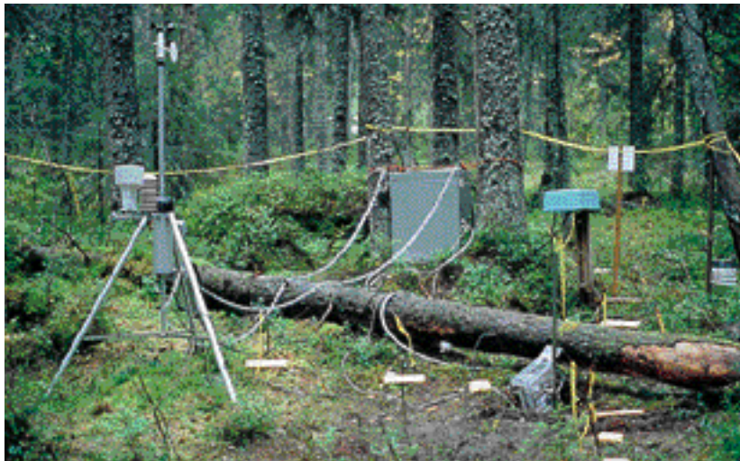
Vaisala's MAWS201 weather station was used for weather conditions monitoring in the field.
