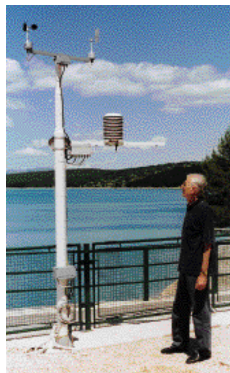
Mr. Branko Grgić stands beside Vaisala's automatic weather station, which is equipped with a QLI50 sensor collector integrated with LabVIEW software.
