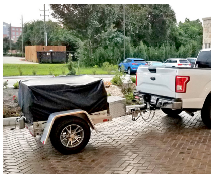
OPT100 Mobile ready to be pulled to a transformer site.
