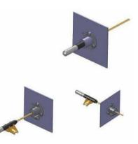
Installation of probe mounting flange
