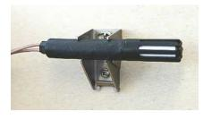
Probe clamp for humidity probe makes installation inside the chamber easy and reliable.
