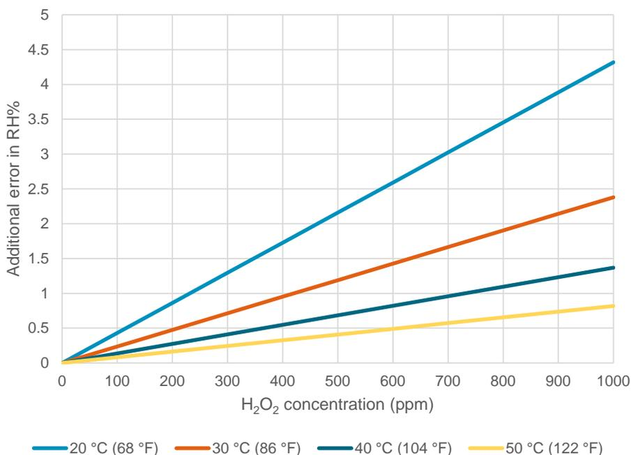
The combination of water vapor and hydrogen peroxide vapor determines the relative saturation (RS). Relative saturation is dependent on the concentration of water and hydrogen peroxide vapor, as well as the temperature of the air. The higher the temperature, the more water and hydrogen peroxide vapor the air can hold. The lower the humidity level, the more H<sub>2</sub>O and H<sub>2</sub>O<sub>2</sub> molecules can be added before condensation.
