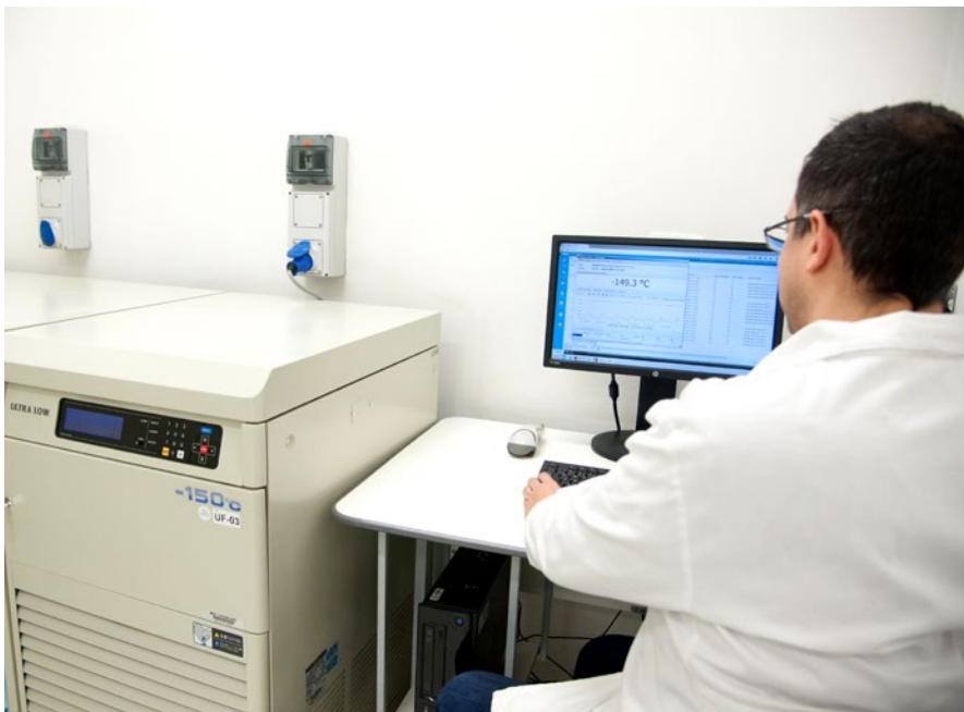
Dr. Motta checking the status of a cryogenic freezer in a viewLinc pop-up alarm window.
