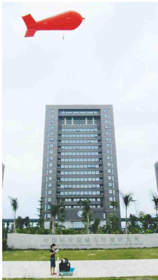
profiles to study the impact of meteorological variables on the vertical distribution of CO<sub>2</sub> in the part of the atmosphere that lies closest to the earth. The sensors were attached to a tethered balloon at a suburban site in Xiamen China, and released to gather data. Xiamen is relevant to this research because the area is undergoing fast urbanization.
