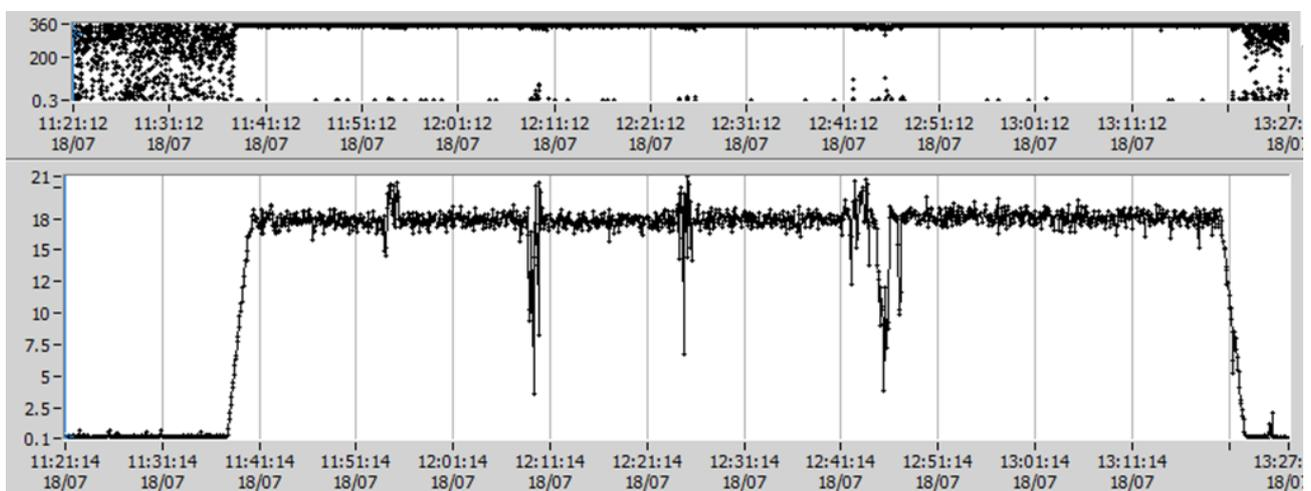
**Figure 8.** Measurement data from the UUT during the test period. Upper graph is wind direction and lower is wind speed. Changes on wind speed value were due to the ice thickness measurements.
