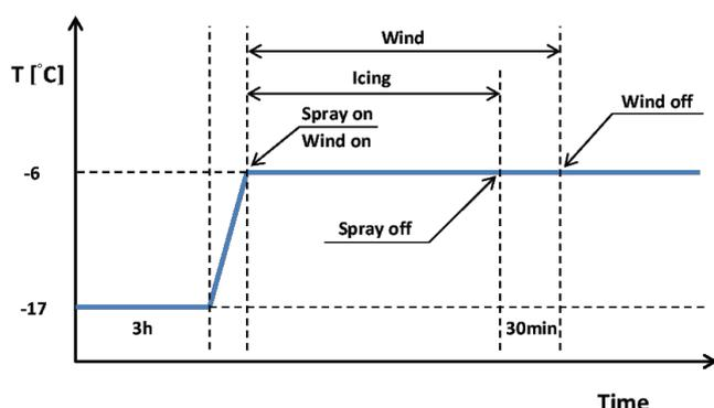
**Figure 1.** Test profile. 1<sup>st</sup> phase is cold soak period, 2<sup>nd</sup> phase is icing period with icing and wind, 3<sup>rd</sup> phase is wind period.
