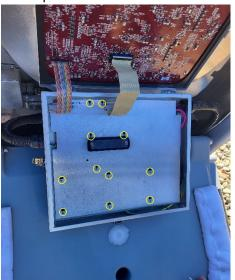
3.) Unhook all cables and ribbons from each of the boards, then remove each component: Linux Board (PN: 610-0037) with SD Card (PN:252672), PC104DSP (PN:510-0001), and Peripheral Board (PN:510-0025)
