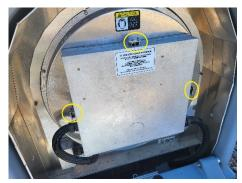
2.) Remove all screws to remove cover panel
