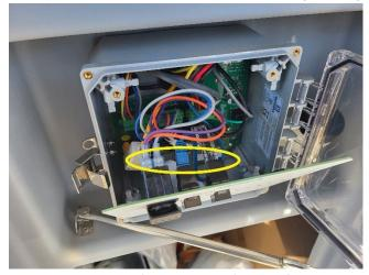
4.) Unscrew and remove the modem carrier (PN: 510-0043) board from control box
