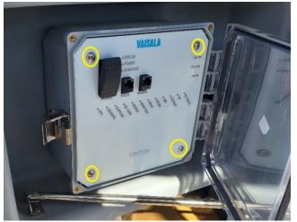
3.) Unplug all of the connections and ribbon cable connected to the operator panel (PN: 610-0024)
