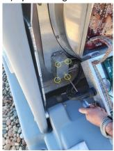
2.) Remove the cables from the inside and unscrew the conduit from the side then remove the four mounting screws to take the Baro off the triton.
