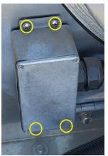
3.) Remove the thermistor (PN:028-0010) by cutting the cable and removing it from the bottom of the solar shade.
