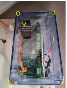
4.) Unplug the connection to the relay (PN: 125-0004), unscrew mounting screws to remove.
