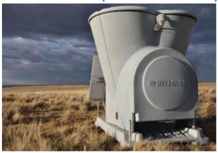
1.) Open the Array Door by stepping on the foot latch
