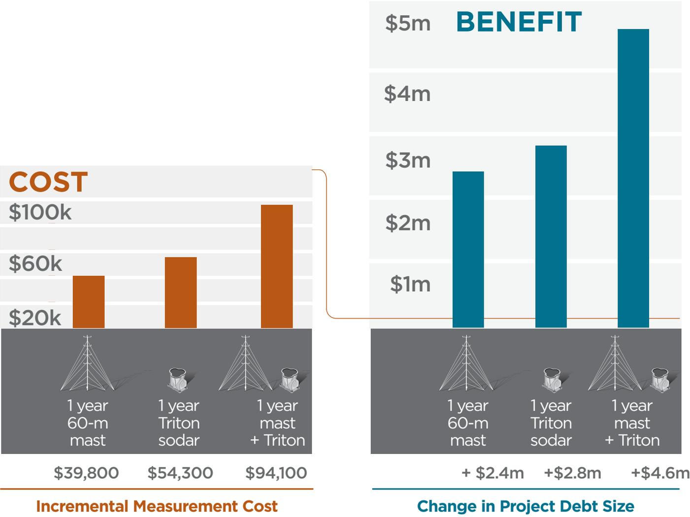
Figure 8: Incremental measurement costs and changes in project debt size, complex terrain scenario
