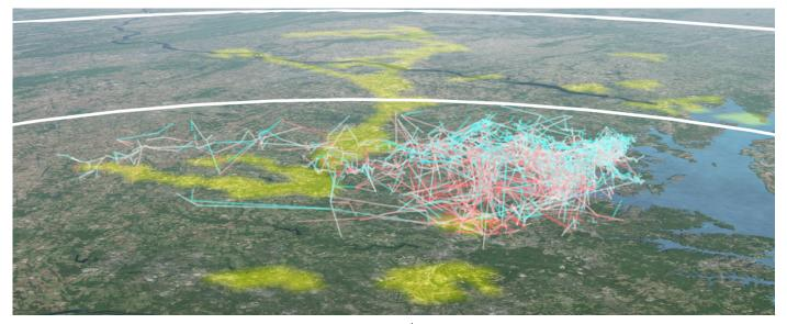
Fig. 4. A screenshot from the DCLMA 3D lightning web application from June 19<sup>th</sup>, 2017 20:05 – 20:10 UTC with GLM flash extents (yellow) added. Positive (red) and negative (blue) LMA sources are clustered into flashes. Range rings of 100 km (lower) and 200 km (higher) from the network center are overlaid.
