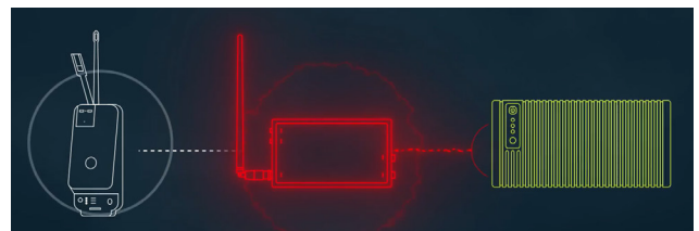
Figure 1: Software-defined radio sending falsified data to receiver
