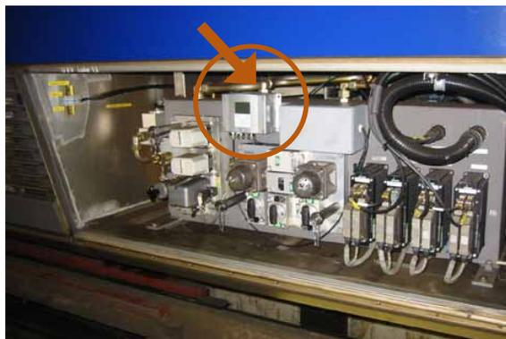
*During the trials the DMT348 was installed in the compressor compartment (in the picture). In the final installation the probe is installed in the compressed air line and the transmitter inside the car, so that the personnel on train can see the alerts.*
