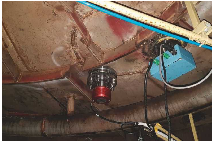
Image 3: Pan bottom showing a refractometer sensor and a microwave meter. Syrup is fed to the pan via a feeding ring.
